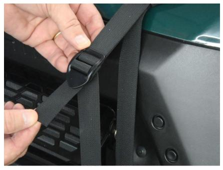
**Step 5:** Before tightening the hood straps, make sure the windshield is square and pulled tight from side to side. Grasp the 8" webbing/loop tabs on either side of the windshield and reposition to center and tighten the windshield as shown below.
