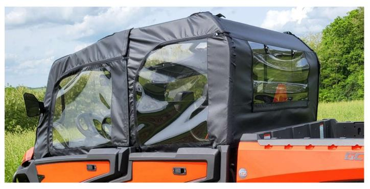
Magnets are sewn into the bottom of the door kit and will attach to the inside of the factory hard door.
