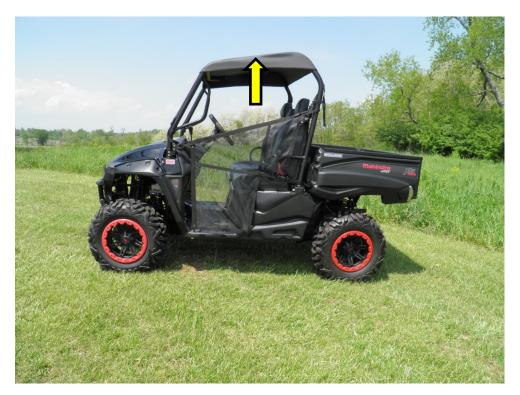
**Step 3:** Place Top Cap loosely on top of the vehicle Roll Bar Cage making sure the Enclosure front visor is facing toward the front of the vehicle. Align Enclosure seams with the center of the roll bars. Pull the Enclosure downward at each Roll Bar post upright to position the Enclosure snug to the Roll Bar Cab frame.
