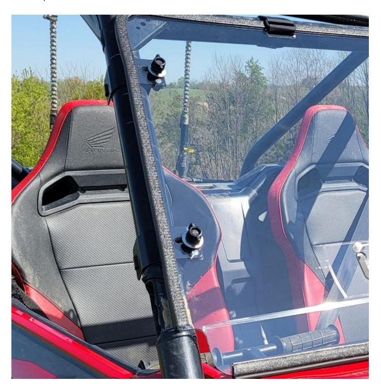
**Step 6:** Use a drill or wrench to tighten the small screws on the back of the clamp. Then twist the bolt assembly more to tighten down the windshield. Do not over tighten! The neoprene washers should not be mashed flat.
