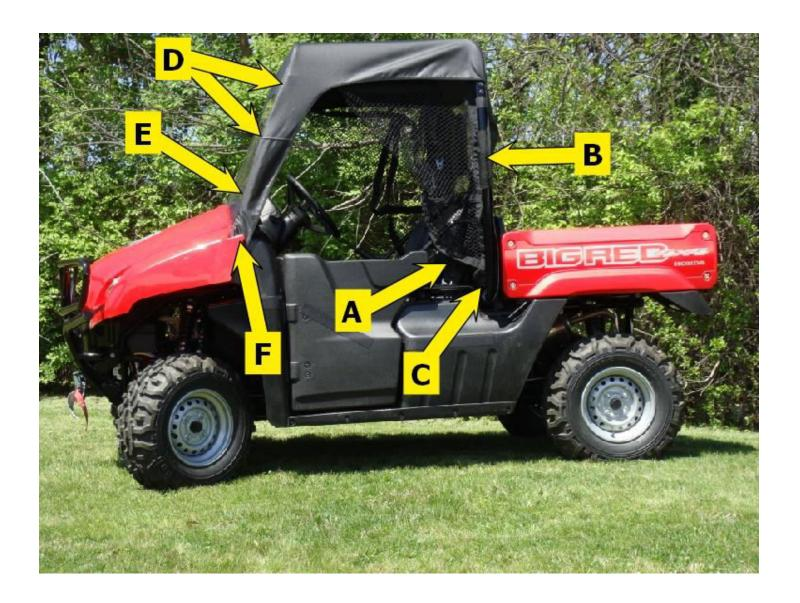
**Step 5:** Begin attaching the back of the enclosure by first squaring the back to the cab frame and attaching the sewn-in Velcro loop at the bottom of the rear panel to the 2 attached 15.5" strips and wrapping the double-sided Velcro straps around the bottom cross bar. Attach the sewn-in Velcro tab to the 2-8" vertical strips near the middle of the back roll bar uprights.
