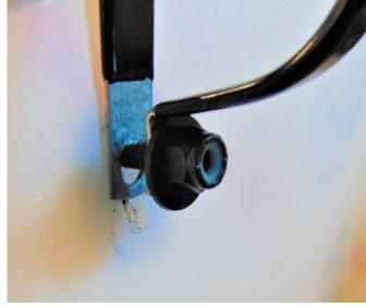
tightened your lock nuts. Over tightening may cause the windshield to crack near the clamp hole.
