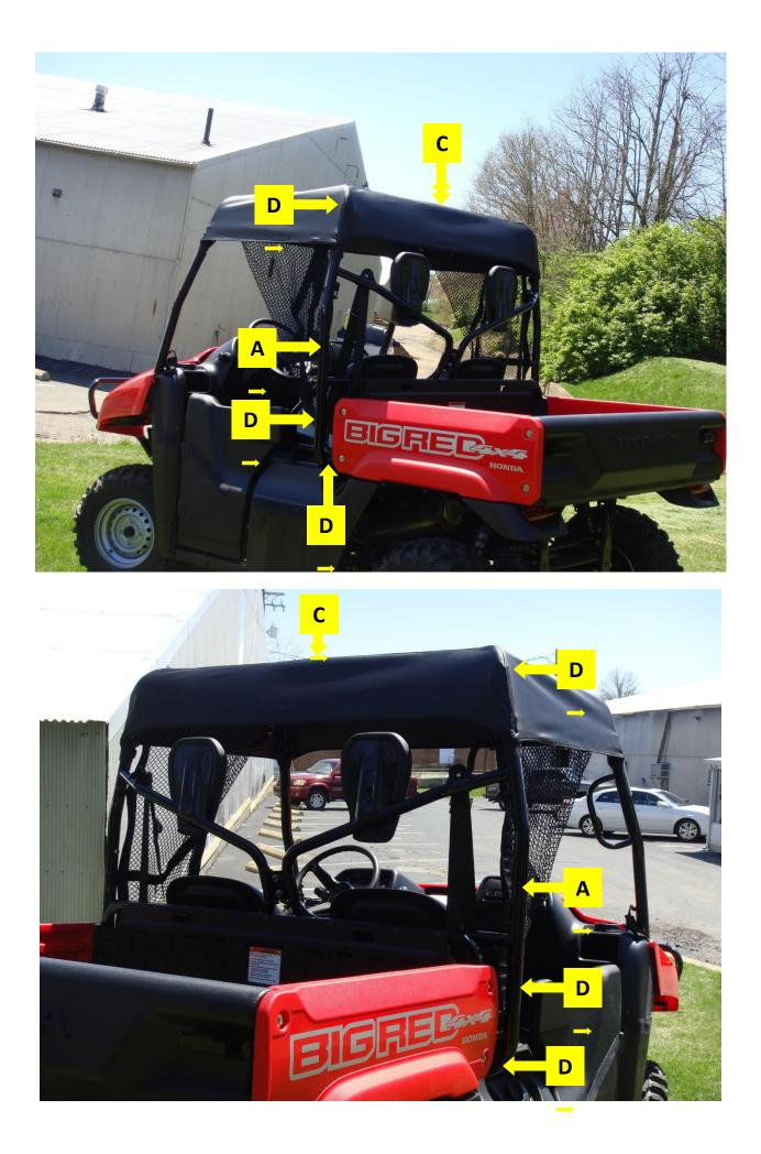
Step 2: Place Rear Window Enclosure on top of Roll Bar Cage and align corner seams with outside center of roll bars.
