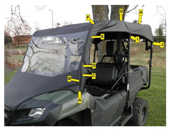
**Step 3:** After all adhesive hook strips are attached, begin attaching the enclosure to the cab frame. As you attach the hook and loop, square each panel to the frame. <u>PLEASE NOTE, FOR MAXIMUM ADHESION, ALLOW THE ADHESIVE</u> <u>HOOK TO ADHERE TO THE FRAME FOR 24 HOURS BEFORE PULLING AGAINST THE HOOK WITH THE LOOP STRIPS.</u>
