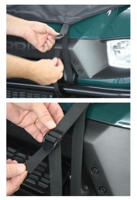
**Step 5:** With the enclosure properly aligned to the cab frame, tighten the front straps by pulling downward from the buckle on both strap ends at the same time as shown.
