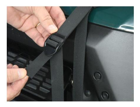
**Step 5:** With the enclosure properly aligned to the cab frame, tighten the front straps by pulling downward from the buckle on both strap ends at the same time as shown.
