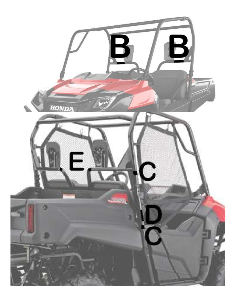
STEP 3: Install polycarb back panel. Insert strap through the outside of the panel, around the roll bar and pull through the plastic clip. Then pull the strap tight and attach it to itself. Do this for all straps.
