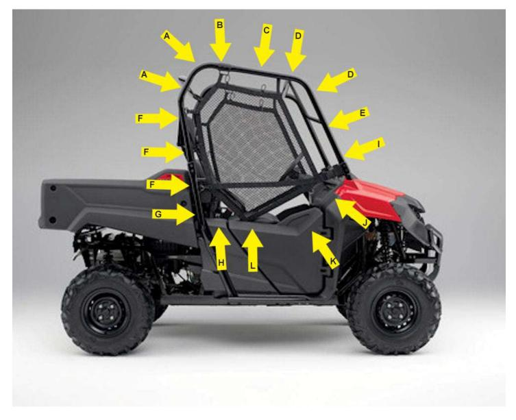
**Step 3:** After all adhesive hook strips are attached, begin attaching the enclosure to the cab frame. As you attach the hook and loop, square each panel to the frame
