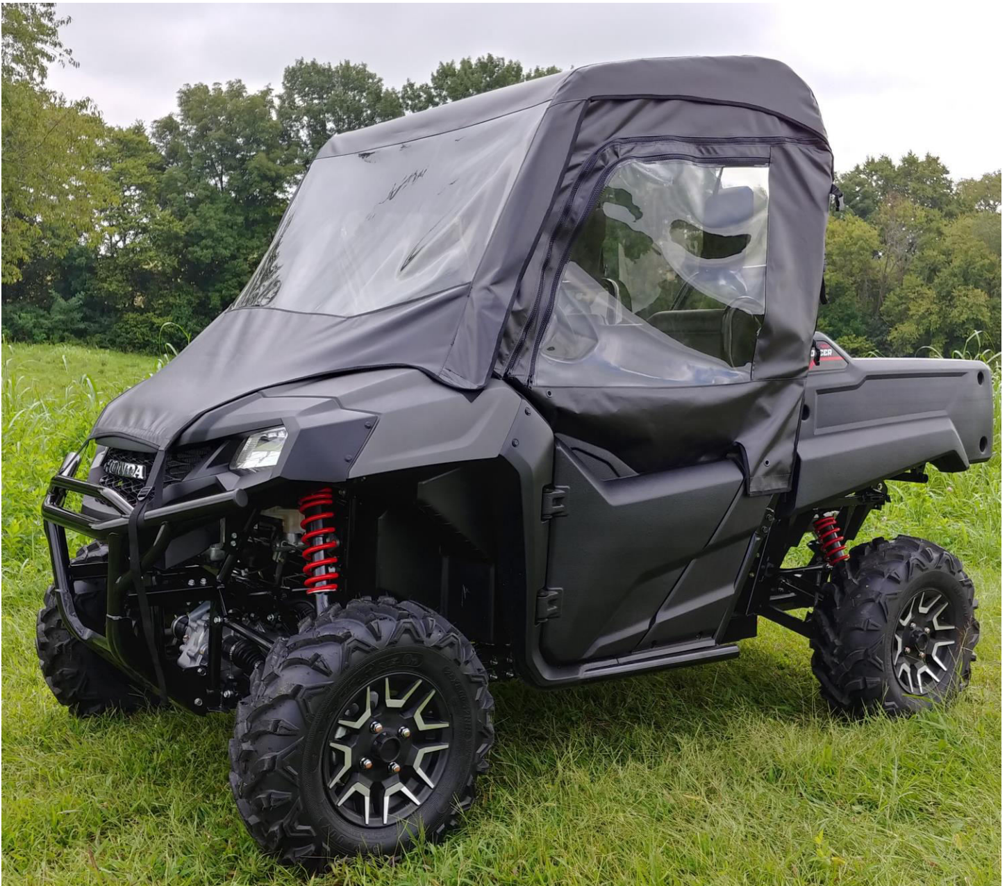
Full Cab Enclosure with Vinyl Windshield Pictured
