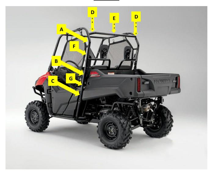
**Step 3:** After all adhesive hook strips are attached, begin attaching the enclosure to the cab frame. As you attach the hook and loop, square each panel to the frame. **PLEASE NOTE, FOR MAXIMUM ADHESION, ALLOW THE ADHESIVE HOOK TO ADHERE TO THE FRAME FOR 24 HOURS BEFORE PULLING AGAINST THE HOOK WITH THE LOOP STRIPS.**
