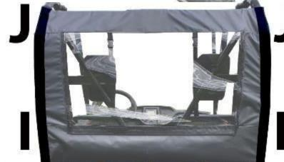
Place these strips toward the inside of the cab. Wrap the tabs around the door and attach to the adhesive Velcro.
