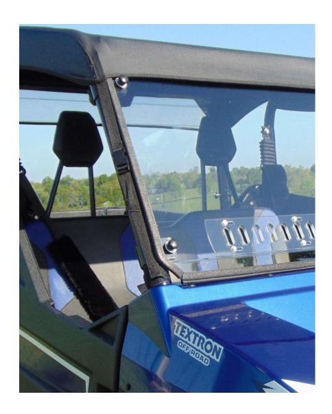
OPTIONAL-Windshield must be installed before completing this step. Unwrap the front two double-sided straps. Remove the adhesive backing from the 49" adhesive hook strip. Adhere the strip to the top of the windshield corresponding to the sewn-in loop in the visor.
