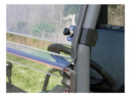
**Step 4:** When satisfied that the bottom windshield section is positioned properly, tighten the two clamps nuts on each clamp.
