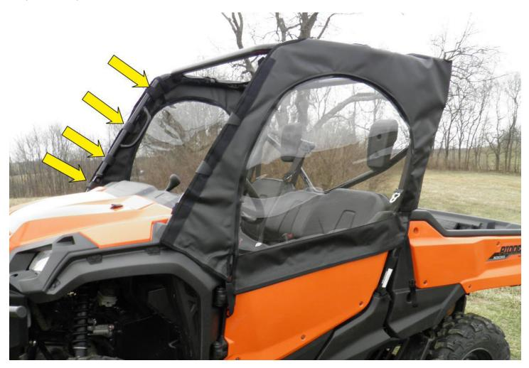
**Step 7**: Double-sided straps are attached to the bottom of the front panel and main door panel. Wrap the straps around the top door hinge and attach the straps to themselves.
