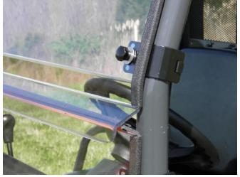
**KNOB BOLTS. NEVER USE THE KNOB BOLTS TO PULL THE CLAMPS TO THE WINDSHIELD.** If the clamps need to be repositioned, loosen the clamp nuts to do so.
