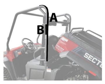
The double sided straps on the back panel will wrap around the roll bar and attach to itself.
