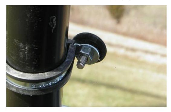
**Step 5:** To mount the upper windshield section, open 2 clamps and wrap around each of the front roll bars.
