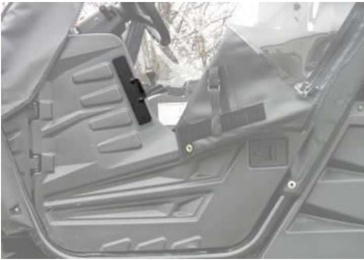
Figure 7: Metal plate has adhesive loop on the back that will attach to the adhesive hook placed on the outside of the factory door.
