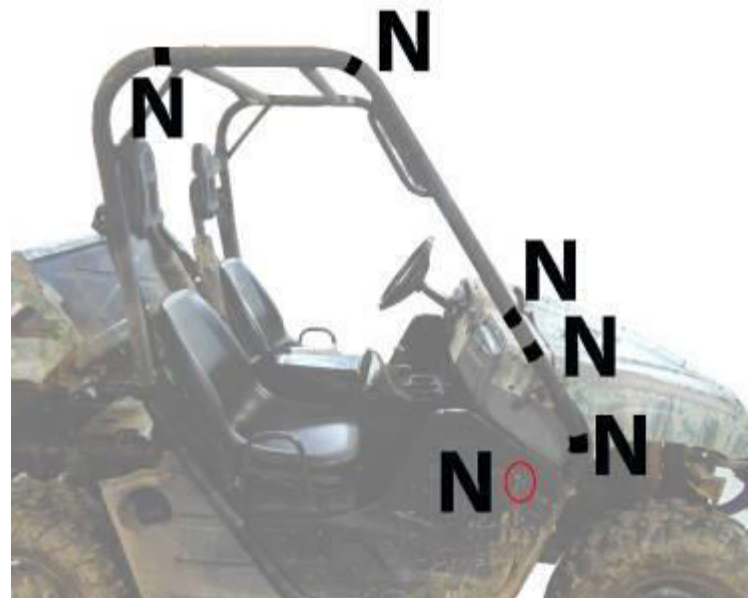
Figure 6: Adhesive strips N will wrap around the bar, the double sided tab for the red circle will not need adhesive Velcro. Wrap this tab around the hinge.
