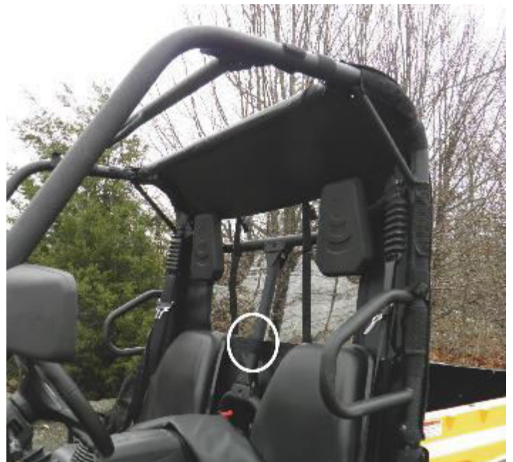
Figure 4: Wrap strip around the back roll bar. Photo also shows placement of Velcro tabs on the sides of the UTV.
