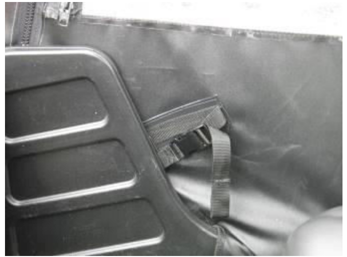
Figure 8: We have included a buckle that will secure the metal plate to the door. If the plate comes loose during use it will stay attached to the door.
