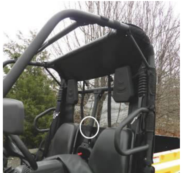
Figure 4: Wrap strip around the back roll bar. Photo also shows placement of Velcro tabs on the sides of the UTV.
