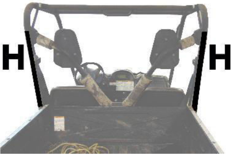
Figure 3: Shows placement of Velcro strips down the back of the roll bar. If you have a back panel the Velcro for this tab is sewn down the back of the back panel.
