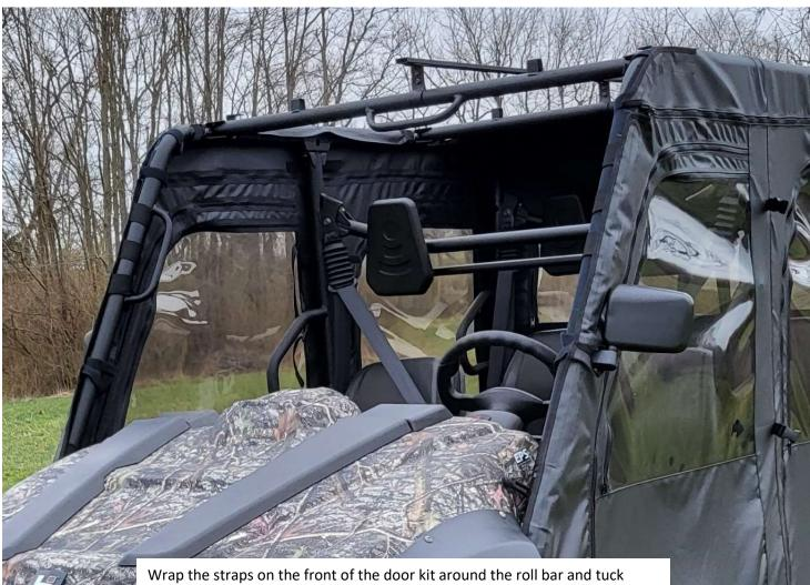
Wrap the straps on the front of the door kit around the roll bar and tuck under the front of the door kit. These straps will attach to the Velcro that you have already installed on the roll bar.
