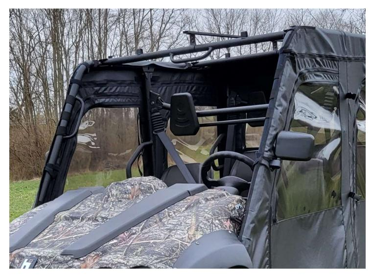
Wrap the straps on the front of the door kit around the roll bar and tuck under the front of the door kit. These straps will attach to the Velcro that you have already installed on the roll bar.
