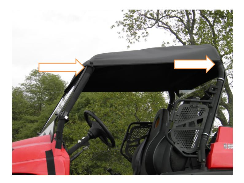
**Step 5:** Align the top as needed to straighten to the frame.
