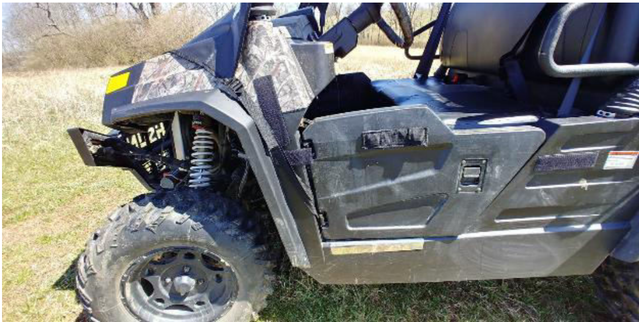
Figure 3: Loop strap around the bottom door hinge, back through the buckle, pull tight.
