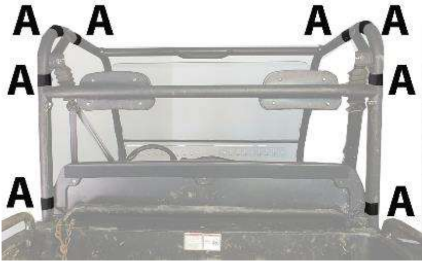
Figure 1: Shows position of Velcro strip A. Wrap tab over the top of the roll bar and attach to the adhesive Velcro strip.
