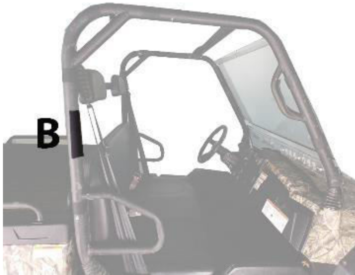
Figure 2: Shows position of Velcro strips B
