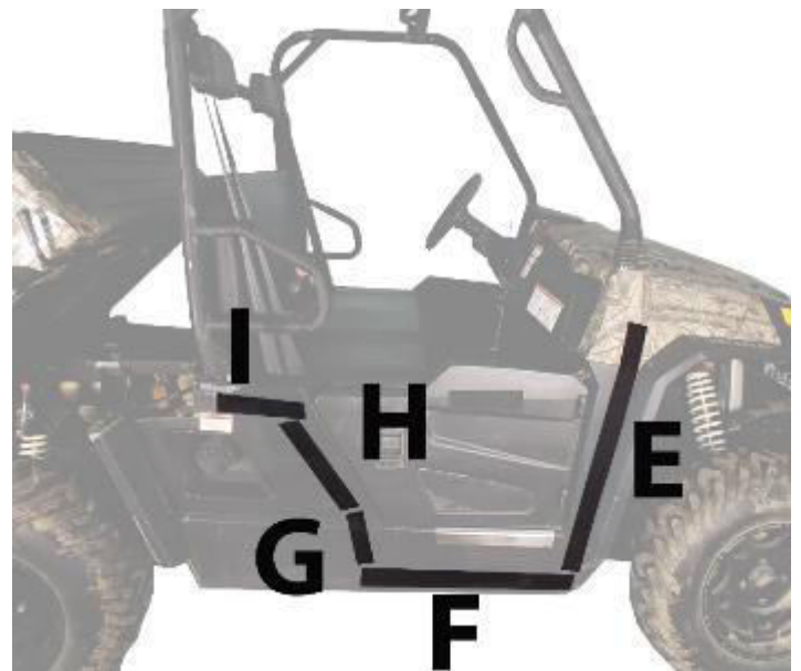
Figure 4: Shows placement of Velcro strips E, F, G, H, AND I.
