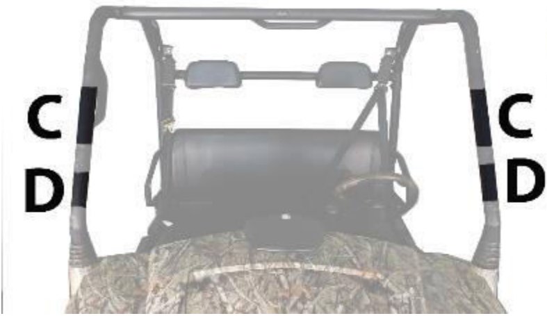
Figure 1: Shows placement of Velcro strips C and D. The tabs on the front of your doors will wrap around the front of the roll bar and attach to the Velcro strip.
