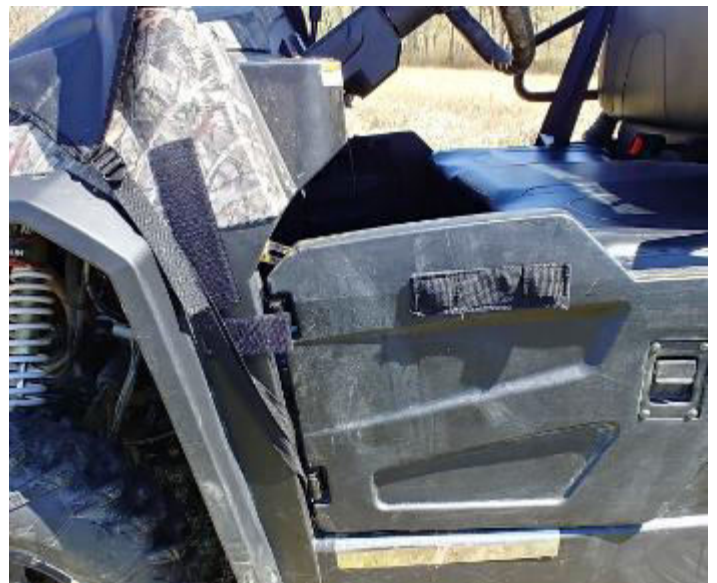
Figure 3: Loop strap around the bottom door hinge, back through the buckle, pull tight.
