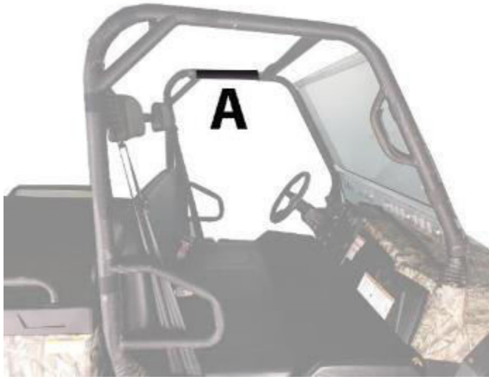
Figure 1: Shows placement of Velcro strips A, place on the top roll bar toward the interior of the cab.
