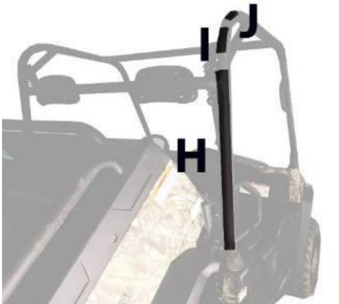
Figure 5: Photo shows placement of Velcro strips H, I and J. If you ordered a door rear window the rear window will have Velcro sewn on the outside of the panel.
