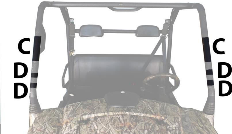
Figure 3: Shows placement of Velcro strips C and D. The tabs on the front of your doors will wrap around the front of the roll bar and attach to the Velcro strip.
