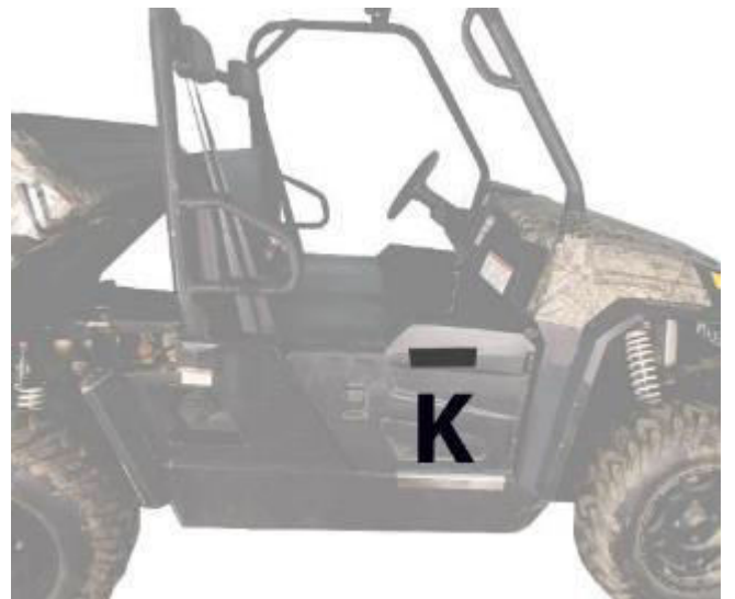
Figure 6: This Velcro strip is for the magnet back attached to the inside of your door.
