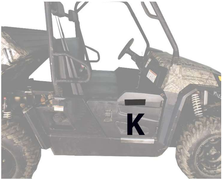
Figure 3: This Velcro strip is for the magnet pack attached to the inside of your door.
