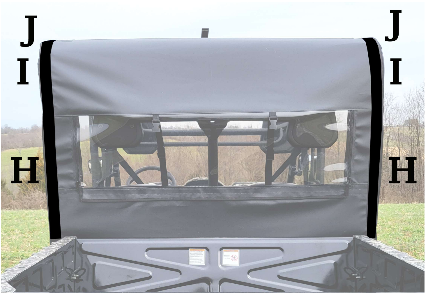
Figure 4: Photo shows placement of Velcro strips H, I and J. If you ordered a door rear window the rear window will have Velcro sewn on the outside of the back panel.
