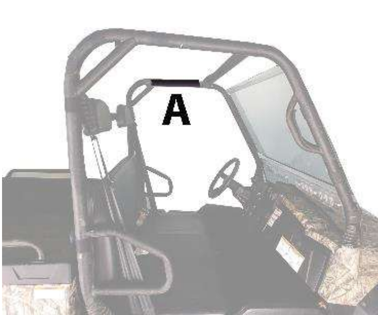
Figure 1: Shows placement of Velcro strips A, place on the top roll bar toward the interior of the cab.
