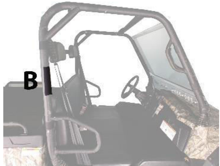
Figure 2: Shows position of Velcro strips B
