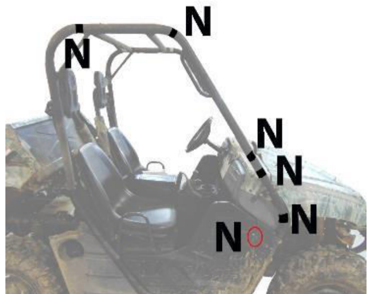
Figure 6: Adhesive strips N will wrap around the bar, the double sided tab for the red circle will not need adhesive Velcro. Wrap this tab around the hinge.
