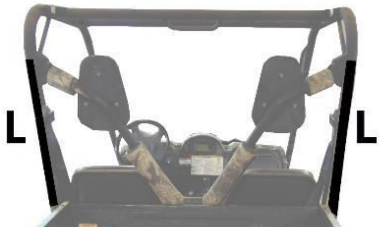
Figure 4: Shows placement of Velcro strips down the back of the roll bar. If you have a back panel the Velcro for this tab is sewn down the back of the back panel.
