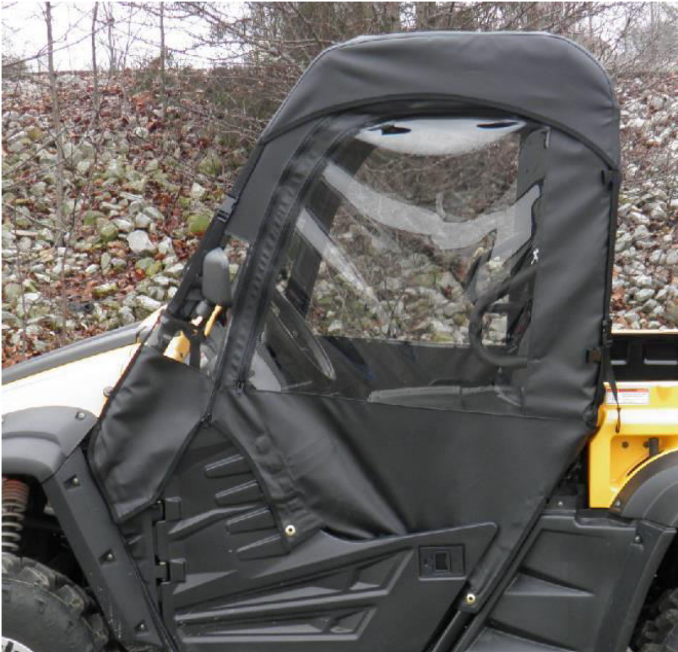
Figure 9: When the installation is complete your door kit should resemble the door kit in the photo.
