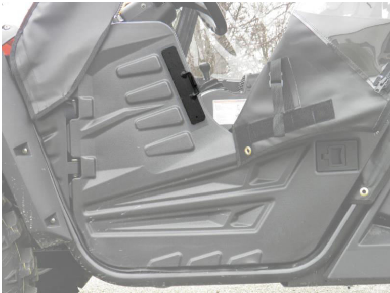
Figure 7: Metal plate has adhesive loop on the back that will attach the adhesive hook placed on the outside of the factory door.
