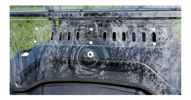
STEP 3: Wrap adhesive Velcro around the roll bar in the vicinity of the clamp holes precut in your windshield. Install loop clamp over the Velcro strip.
