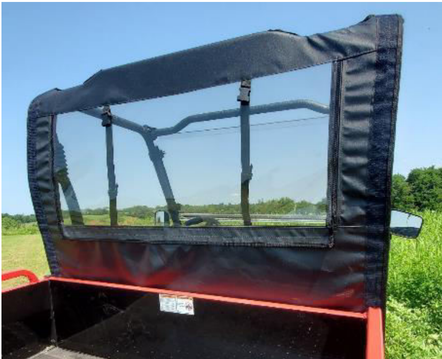
Figure 3: There are double sided straps on either side of the back panel, you may choose to use Velcro here for extra hold but this is not necessary. Wrap these straps around the bar and attach double sided straps.
