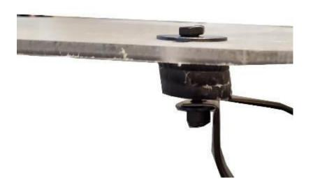
Photo to left shows the order of hard ware. Bolt, large washer on top, through lexan, 3 spacers on the flat part of the loop clamp, with small washer and lock nut on the bottom.
