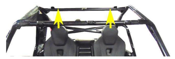
Attach loop clamp to roll bar open end facing the inside of the utv. Flat side facing up. Drill through the top of the lexan and through the hole in the loop clamps. stack three lexan spacers between the hard top and the loop clamp. Insert bolt and large washer through the top of the lexan and through the spacers and through the hole in the loop clamps. Secure with small washer and lock nut.
