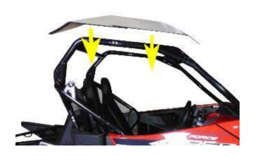
Set assembled hard top on top of roll cage. Small piece goes to the back.
