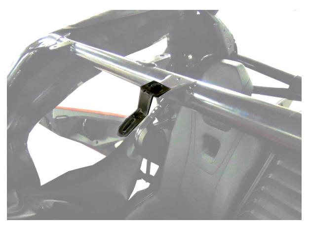
**Step 9:** Line up the slot of the bracket with the hole in the windshield. Insert bolt and large washer through the outside of the windshield and through the slot in the metal bracket. Secure with washer and lock nut. You may now fully tighten all lock nuts into place. Take care not to over tighten the lock nut attached to the windshield.
