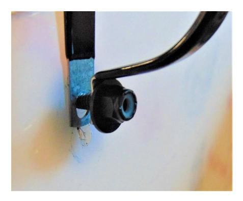
Small washer and lock nut are positioned on the inside of the utv.
