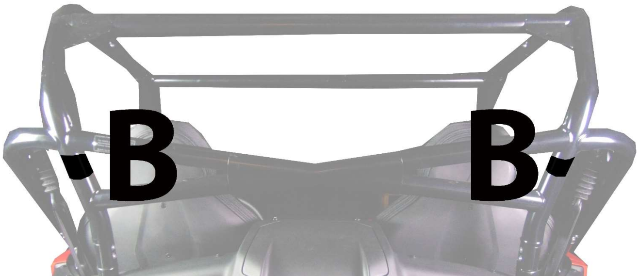
Figure 2: WRAP THESE VELCRO STRIPS AROUND THE ROLL BAR AND ATTACH DOUBLE-SIDED STRAPS.
