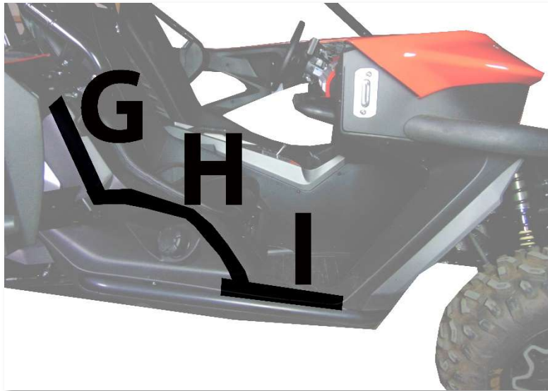
Figure 5: SHOWS PLACEMENT OF VELCRO STRIPS (G, H AND I) STRIP H MAY NEED TO BE TRIMMED IN ORDER TO FOLLOW THE CURVE OF THE UTV.
