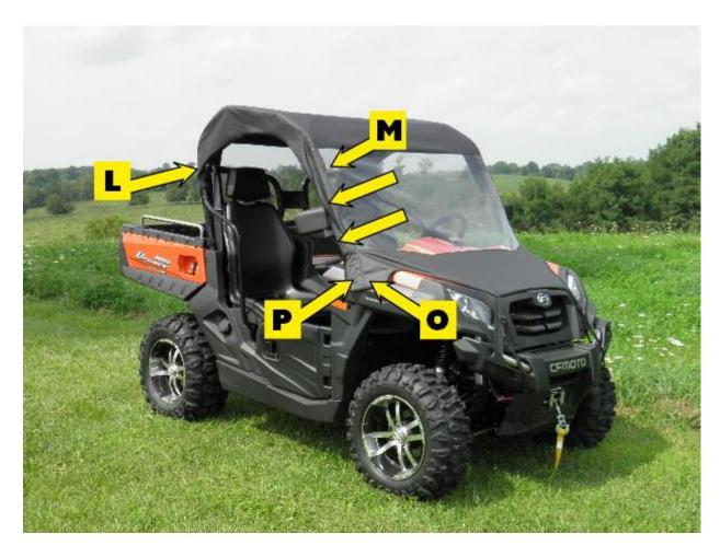
**Step 3:** After all adhesive hook strips are attached, begin attaching the enclosure to the cab frame. As you attach the hook and loop, square each panel to the frame. **PLEASE NOTE, FOR MAXIMUM ADHESION, ALLOW THE ADHESIVE HOOK TO ADHERE TO THE FRAME FOR 24 HOURS BEFORE PULLING AGAINST THE HOOK WITH THE LOOP STRIPS.**
