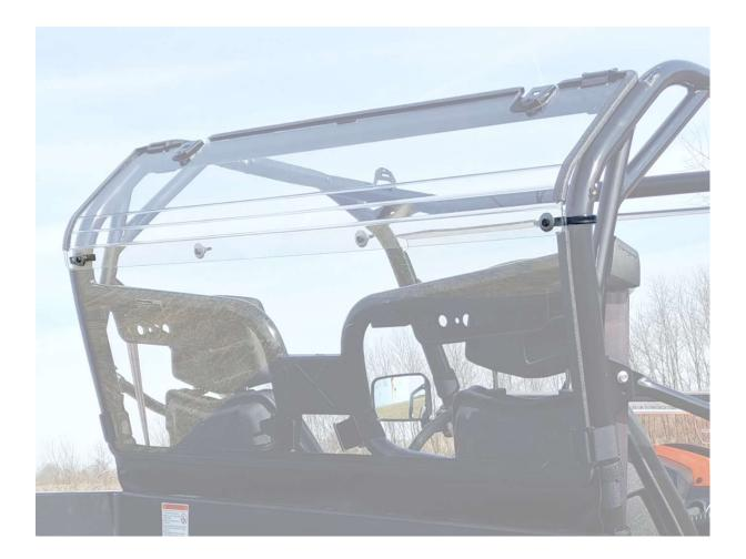
**Step 9:** When satisfied that the back panel is positioned properly, tighten straps and nuts on each clamp.
