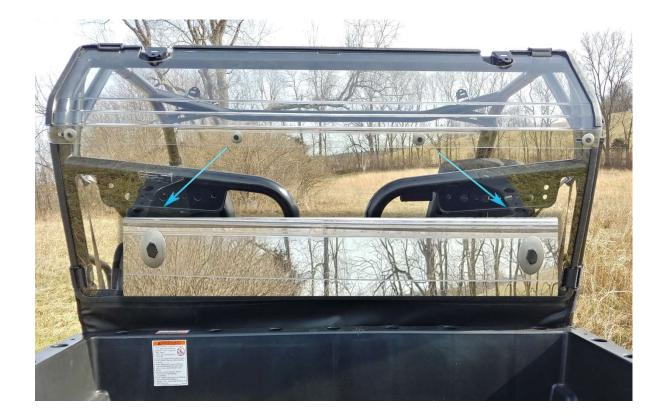
**Step 3:** Pull the protective paper for the edges of the two pieces of lexan and use the two bolts and hardware (bolt – neoprene washer – metal washer – lock nut) to assemble top and bottom pieces of back panel (reference below)
