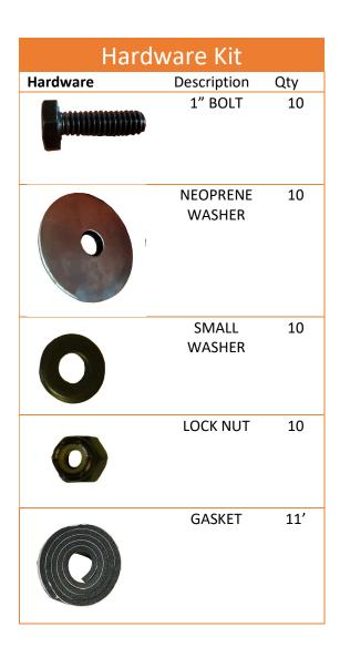
**STEP 2**: Connect the two pieces, the front piece will overlap the back piece. Use a neoprene washer and bolt, through the top of the front piece, through the back piece, secure with small washer and lock nut. Push the bolts through the gasket to create a watertight seal.
