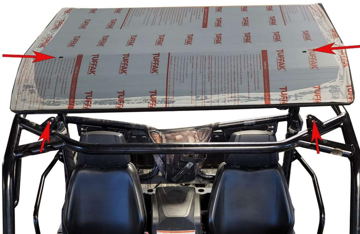
**STEP 7:** Peel back protective paper to reveal the holes in the hard top. Insert bolt and neoprene washer through the top of the hard top and through the holes in the welded-on metal tabs. Secure with small washer and lock nut. Hand tighten only at this time.
