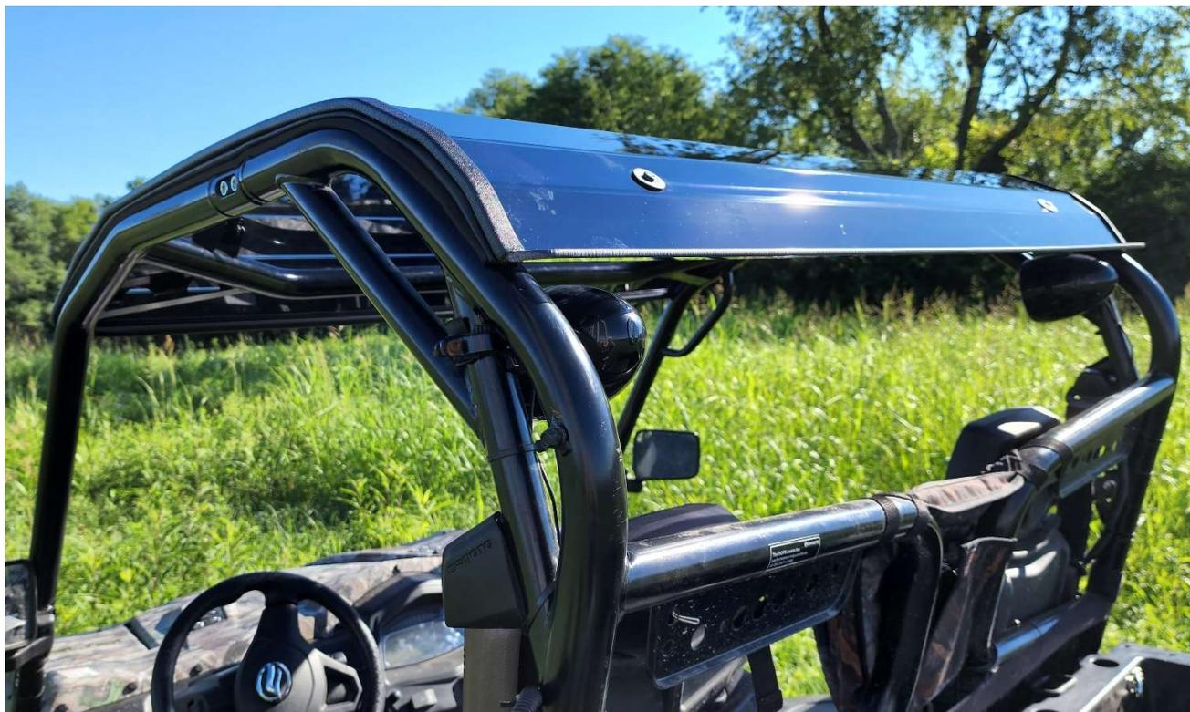
**STEP 6:** Line up holes pre-cut into the hard top with the holes in the welded-on tabs on the top roll bars.
