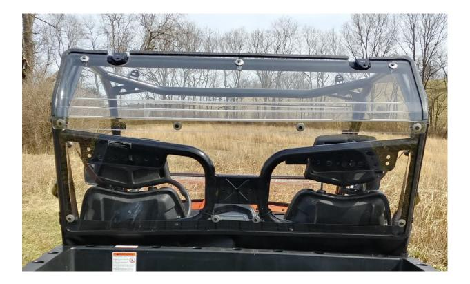
**Step 3:** One at a time, open a clamp and wrap around the rear roll bars corresponding to the picture shown below. The flat side of the loop clamps should face forward with the bolt hole openings on the inside of the roll bars.
