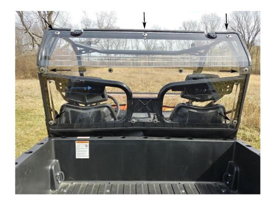
**Step 6:** When satisfied that the back panel is positioned properly, tighten the nuts on each clamp.
