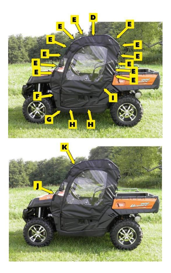
**Step 3:** After all adhesive hook strips are attached, begin attaching the enclosure to the cab frame. As you attach the hook and loop, square each panel to the frame. <u>PLEASE NOTE, FOR MAXIMUM ADHESION, ALLOW THE ADHESIVE</u> <u>HOOK TO ADHERE TO THE FRAME FOR 24 HOURS BEFORE PULLING AGAINST THE HOOK WITH THE LOOP STRIPS.</u>
